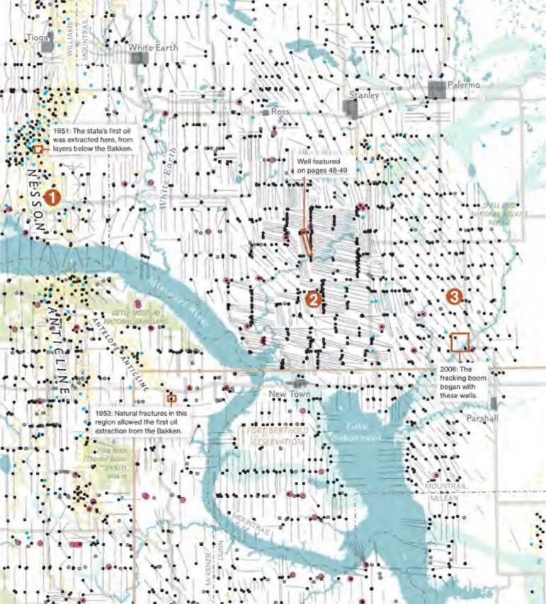
NESSON ANTICLINE Early traditional drilling, in the 1950s, focused on this north-south strip, where reservoirs of oil are trapped along an arching geologic structure called an anticline.
